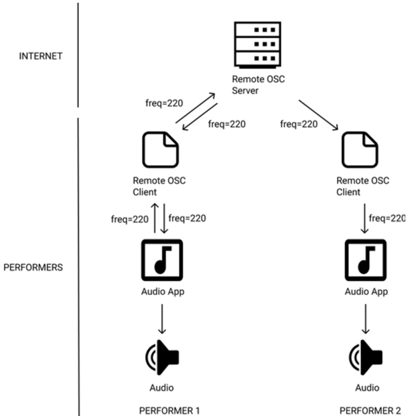
**Figure 3** A typical use of Remote OSC in a networked ensemble. Performer 1 sends freq=220 data which will be received by all members
